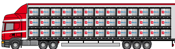
Hintransport (Mega-Trailer): 78 beladene ID PACK-Systeme (1225 x 825)
