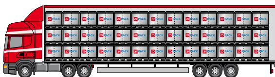
Transport to destination (mega trailer): 78 fully loaded ID PACK containers (1225 x 825)
